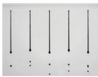
Ink drop formation on the journey from printhead to substrate. To achieve the best image quality Onset must fire a drop at the print surface to land with pinpoint accuracy and in perfect shape. Only good ink design, tuned to the printhead, makes reliable jetting possible.
